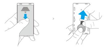
After factory setting, RM433R2 remote controller is bound to iFan04 by default. Simply remove the battery insulation sheet to use. If the device connected to iFan04 is not controlled by the remote controller, try to learn the remote controller again.
