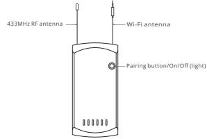
① The device weight is less than 1 kg. The installation height of less than 2 m is recommended.
